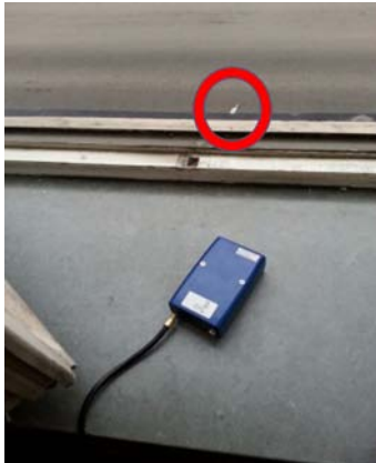
Figure 4, Aethalometer measuring C_{\text{BC},\text{out}} at Artillerigatan with red ring marking the inlet of the hose sticking out through the porthole.
