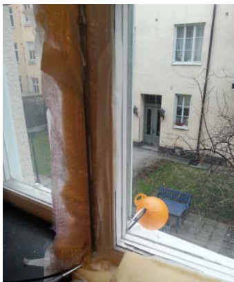
Figure 5, Hoses for outdoor monitoring sticking out through the provisionally closed window at Grevgatan.
