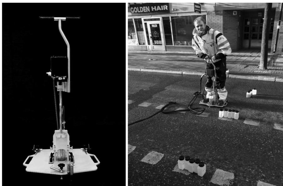
Fig. 2. The VTI wet dust sampler (WDS II). Front view (left) and sampling in a city street (right).
