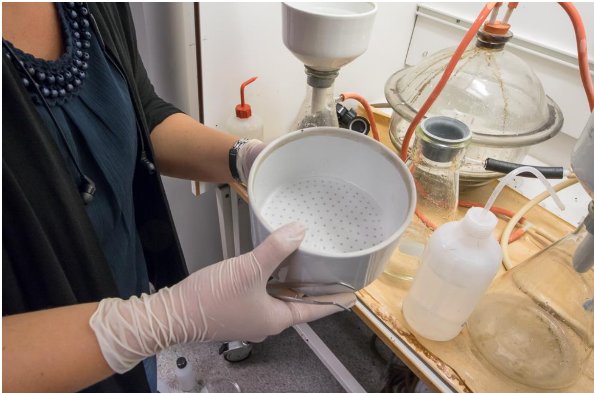
Buchner funnel with Munktell 00H filter for filtering samples
