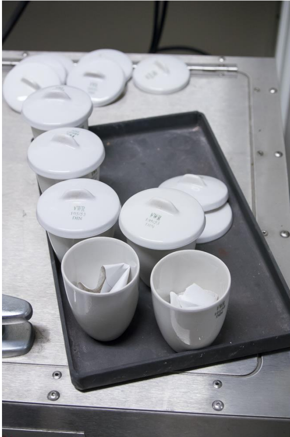
Filters prepared in pots for burning
