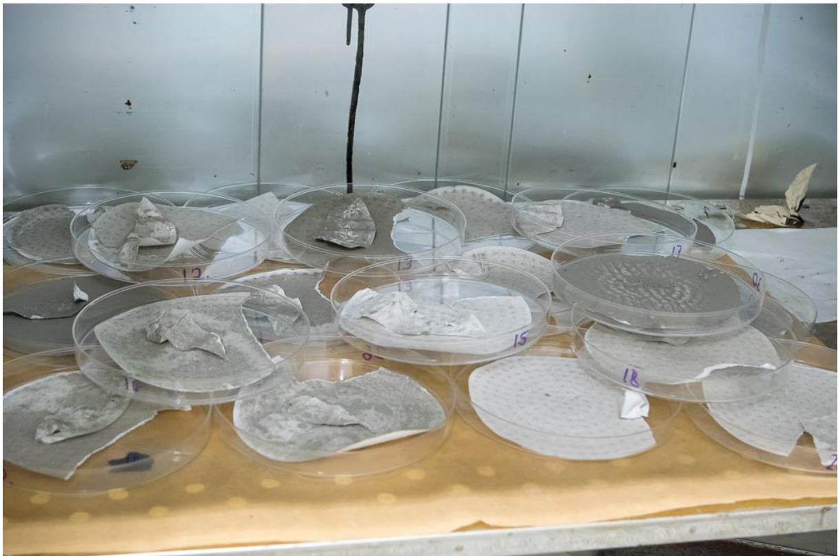
Drying of filters before weighing
