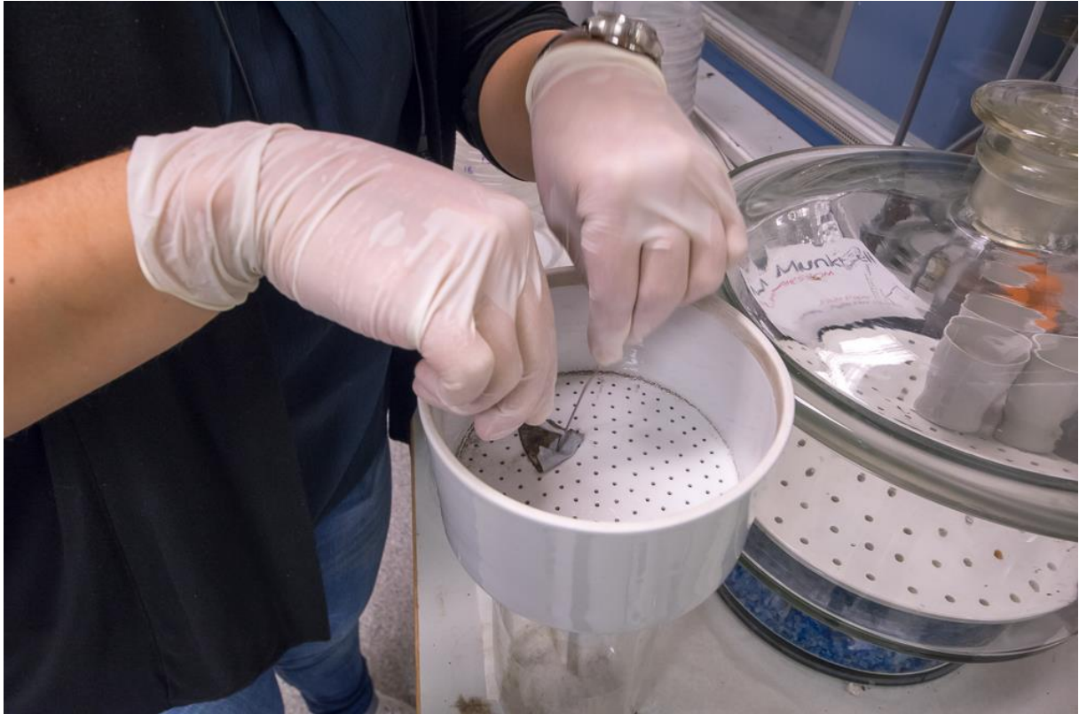
Picking up residual dust from funnel
