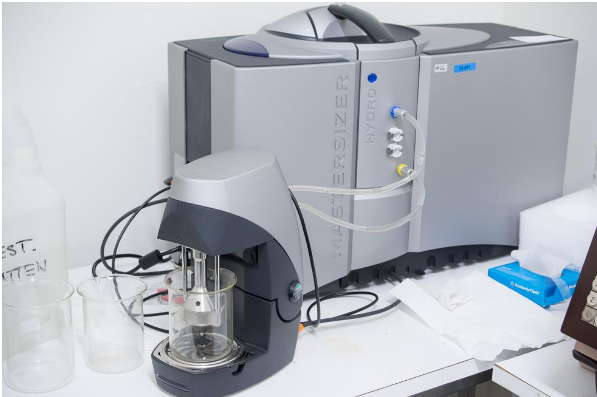
Malvern Master sizer for particle size distribution analysis
