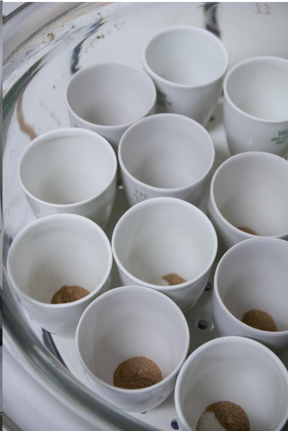
Burnt filters with residual non-organic material
