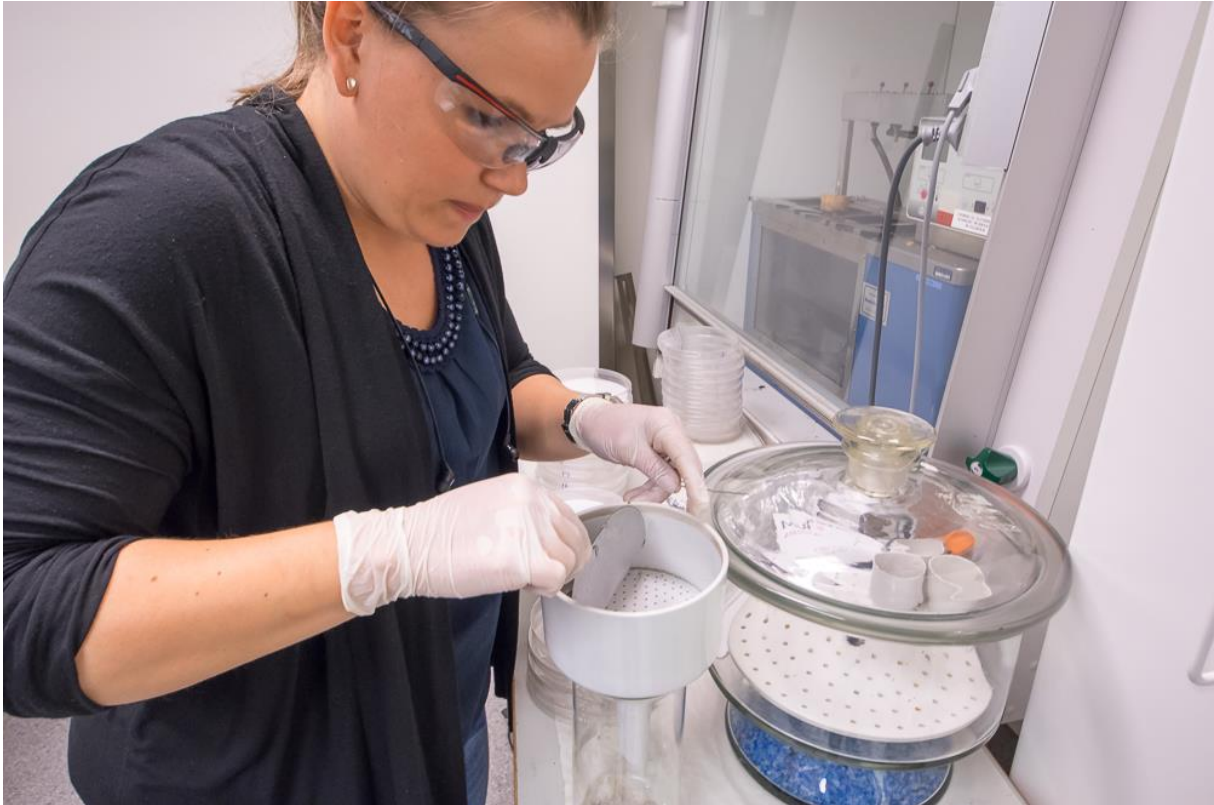
Removing filter from funnel.
